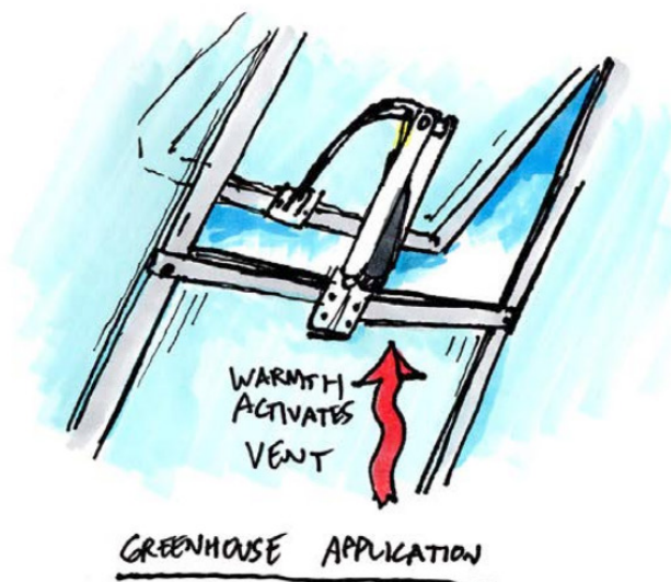
Figure 4: Action of thermal actuators in response to heat load. A typical greenhouse application is depicted on right, where the load of the window causes the actuator to retract as it cools.
