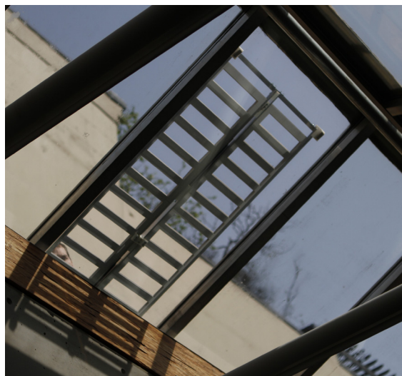
Figure 12: The completed prototype placed in position on the test site. Bottom Left: Temperature above 20°C (59°F). The ambient air temperature closes the shutter and limits solar gain. Unfortunately, Vancouver has not had a sunny day in over two weeks at this point. Bottom right: Apparatus installed, visible from below. Temperature below 15°C (59°F).
