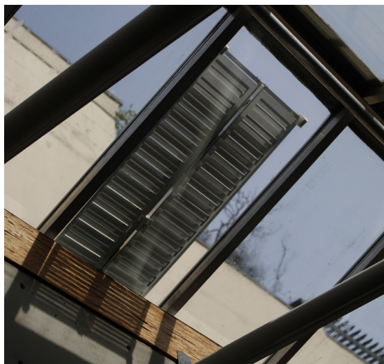
Figure 12: The completed prototype placed in position on the test site. Bottom Left: Temperature above 20°C (59°F). The ambient air temperature closes the shutter and limits solar gain. Unfortunately, Vancouver has not had a sunny day in over two weeks at this point. Bottom right: Apparatus installed, visible from below. Temperature below 15°C (59°F).
