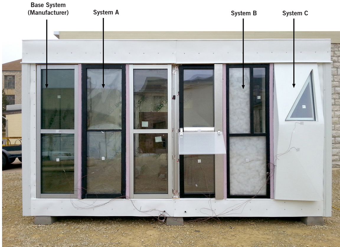
Figure 1: Image showing test structure and 1:1 scale prototypes constructed by the students for thermal testing.
