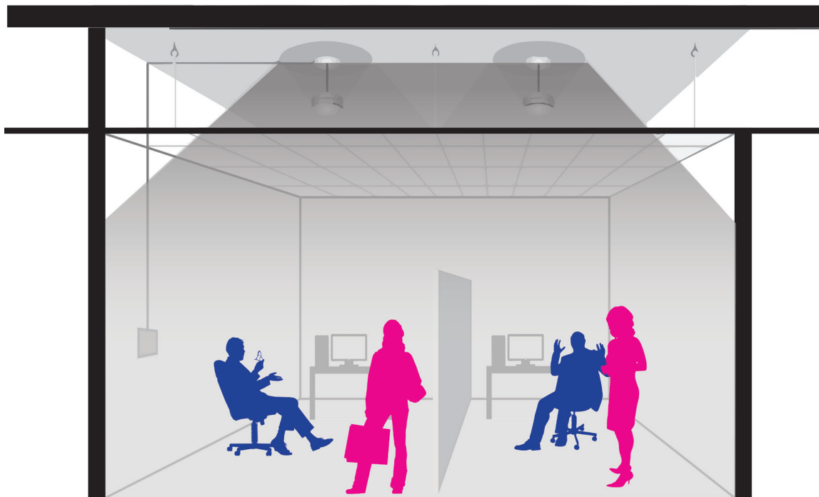
Figure 1: Conventional sound masking system in suspended acoustical ceiling (Courtesy of Environmental Acoustics Inc. © 2014 K.R. Moeller Associates Ltd).
